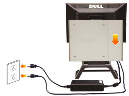
8 Connect the power cables to an outlet. Install the cable cover
